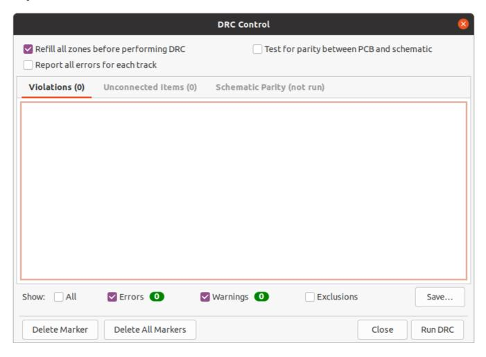
The top section of the DRC Control window contains some options that control the design rule checker:
