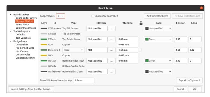
Set the number of copper layers in the upper left corner and then enter the physical parameters of the stackup if desired. These parameters may be left at their default values, but note that the board thickness value will be used when exporting a 3D model of the board. If you plan to use this feature, it is a good idea to ensure that the stackup thickness is correct.
