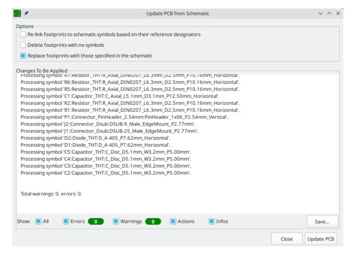
The tool adds the footprint for each symbol to the board and transfers updated schematic information to the board. In particular, the board's net connections are updated to match the schematic.
