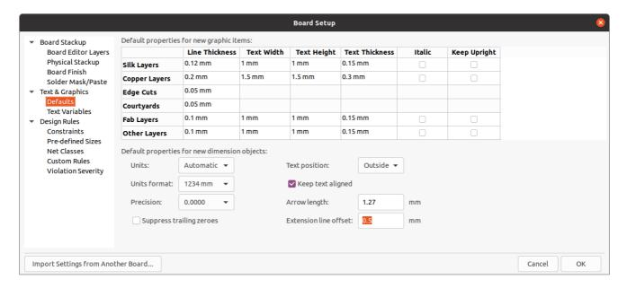
Line thickness, text size, and text appearance can be configured for the six different categories of layers shown in the dialog. Additionally, the properties for dimension objects can be configured for all layers. For more details about dimension properties, see the Dimensions section below.
