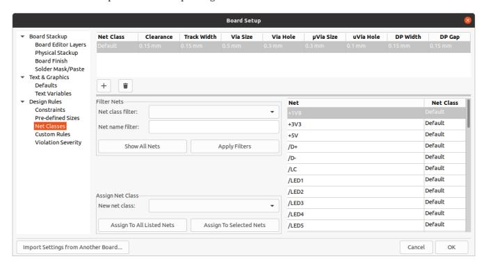
The upper portion of the Net Classes section contains a table showing the design rules that apply to each net class. Every class has values for copper clearance, track width, via sizes, and differential pair sizes. These values will be used when creating tracks and vias unless a more specific rule overrides them (see Custom Rules below).
